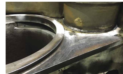
Above: Detail of the cast steam port welded to the fabrication.
