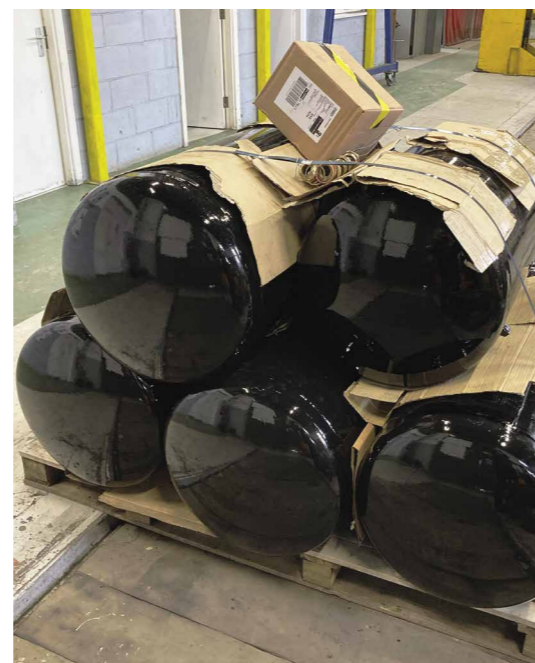
The cylinders were then primed, painted and palletised ready to send back to LMS.
