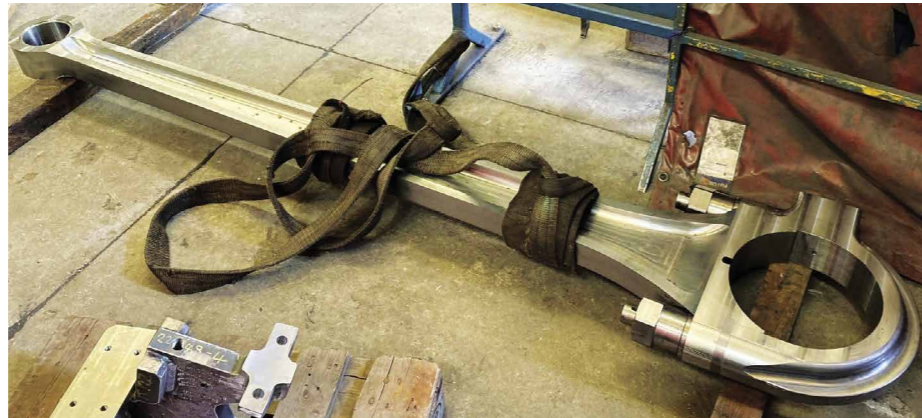
The newly machined inside connecting rod.
