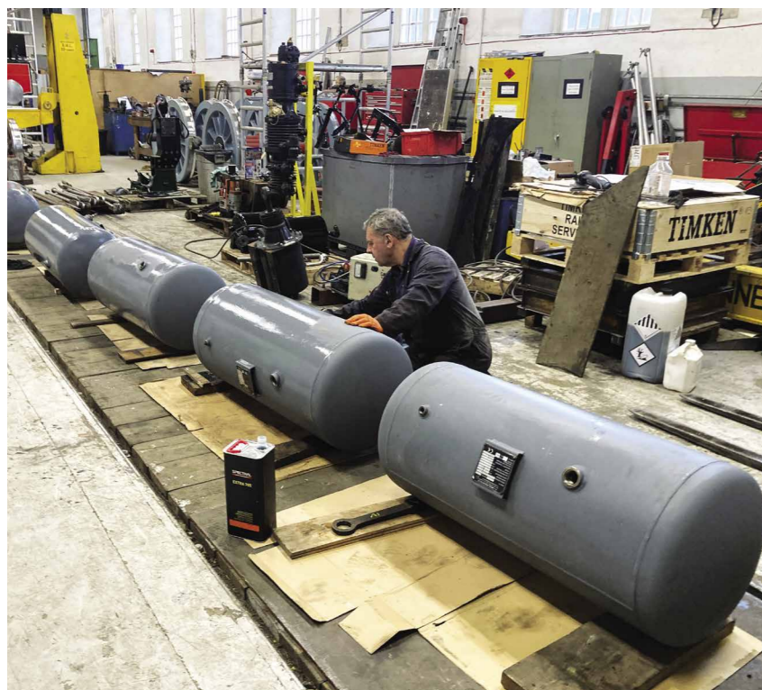
The cylinders were then primed, painted and palletised ready to send back to LMS.
