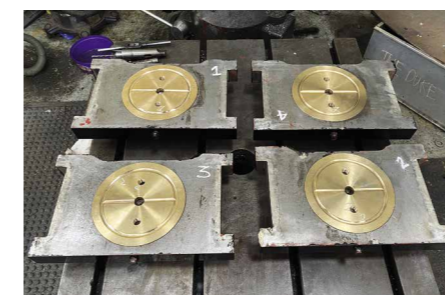
Ian Greenan machined new tender slipper block pads.
