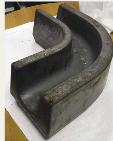
A foundation ring corner awaiting machining.
