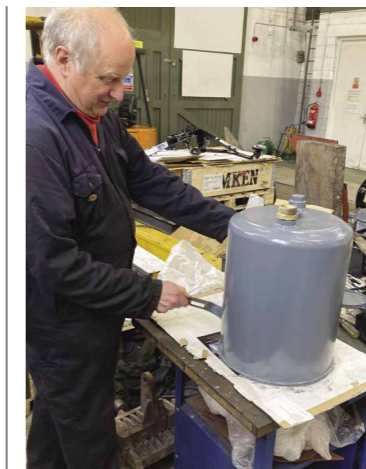
Top right: The reversing stand has been fully dismantled for inspection and repairs and George Bee is seen applying some paint after the first stage reassembly.
