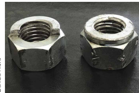
A one-inch Philidas nut showing the failure.
