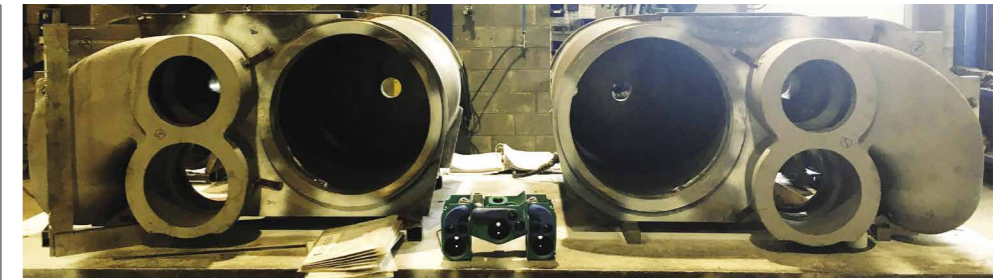
The two outside cylinders seen from the front with David Elliott's 1/8 th scale model between them.
