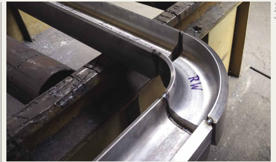
A corner tacked in place awaiting final welding.
