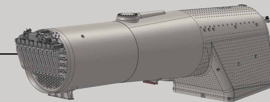
Diagram 118b boiler drawing shows fitted with Melesco type superheater header as used on Tornado .
