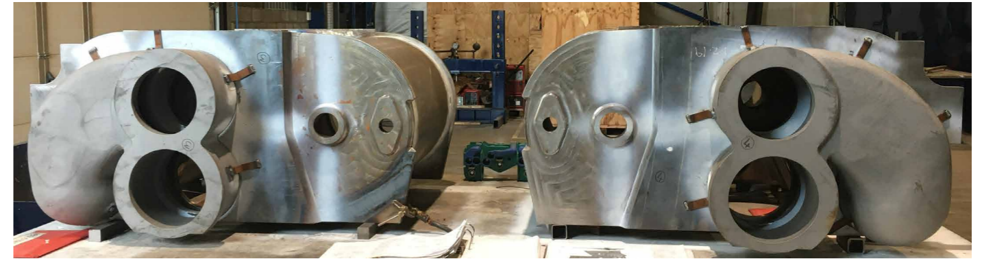
Above: The two outside cylinders seen from the rear.
