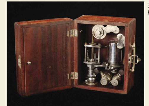
A Crosby 'marine' type indicator gauge of the sort used by the LNER.
