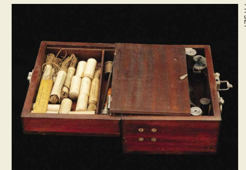
The contents of the small compartment, indicator rolls and instruments.
